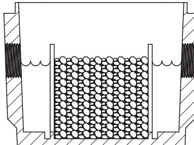
**INSTALL A AND B FILTERS IN ALTERNANCE STARTING FROM THE INLET SIDE AND WITH AN "A" FILTER.**
